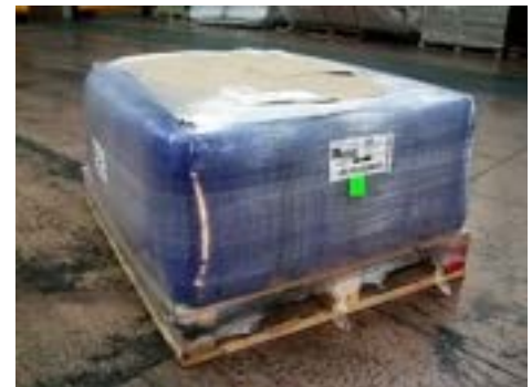
Drums, tied down and properly wrapped
