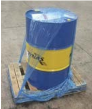
This drum is barely secured.
